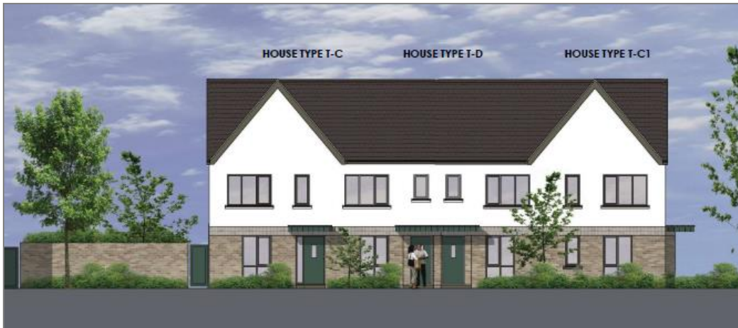
Figure 2.16 House Types T-C, T-D and T-C1 at Tanner Lane. Note the brock and self-coloured render finish.
