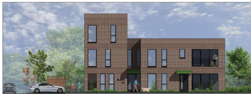
Figure 2.23 Duplex Block F-R at Flemington Lane, note the brick and light coloured sone finish, glazed balconies and pressed metal canopy over the front door.
